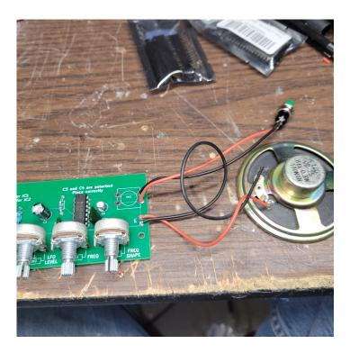
This kit wasn't originally designed to go in a case - it was to teach soldering, and to show a simple circuit. If you want to put this in a case, you might want to "fly" the components off the board. It's simple - rather than putting the components directly on the boards, you can put them at the ends of wires inserted into the board like this picture. You can do the same thing with the potentiometers, if you want to make a nice case for this.
