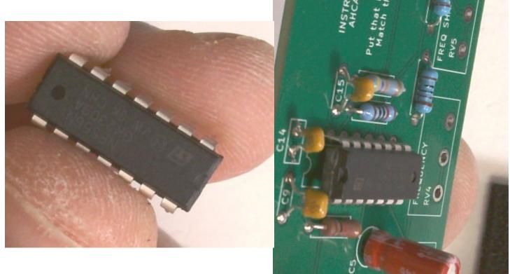
Step twenty: Caution - this is another component that can be put in backwards. Find the 555 timer - there will be two of them. These are placed at U2 and U5. Again, make sure to match the notch. Place, solder. No need to clip. You may have to push in the legs a bit to get them to fit.
