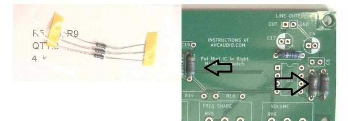
Step nine: Bend, place, solder, and trim the ends for R6,R7. These are 6k2 resistors with color bands Blue,Grey, Red,(tolerance).
