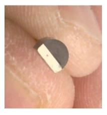
This is how the transistor should be placed. Place, solder, and clip.
