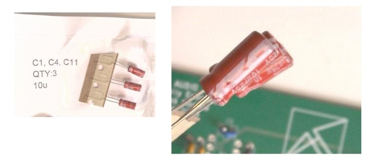
See how the white stripe is matched to the white half of the silkscreen - all of the electrolytic capacitors need to be matched in this way. Place C1,C4,C11 - 10u - the right way round - and solder, and trim.
