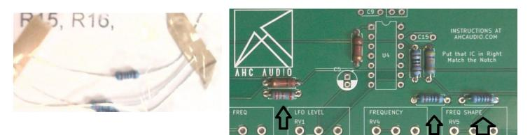
Step eleven: STOP THIS COMPONENT CAN PHYSICALLY BE PLACED IN TWO WAYS,BUT ONLY WORKS ONE WAY ELECTRICALLY FOLLOW THESE INSTRUCTIONS TO THE LETTER.
