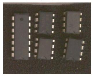
Find the 14 legged bug - it will be labeld 556 - it might be NE556 or LM556. Place on the board at U4 making sure that you match the notch. See the below picture. You might use a little bit of tape to hold it in place while you solder. You might have to squeeze the legs in to get them to fit in the PCB. You place and solder, but you don't need to clip the wires.
