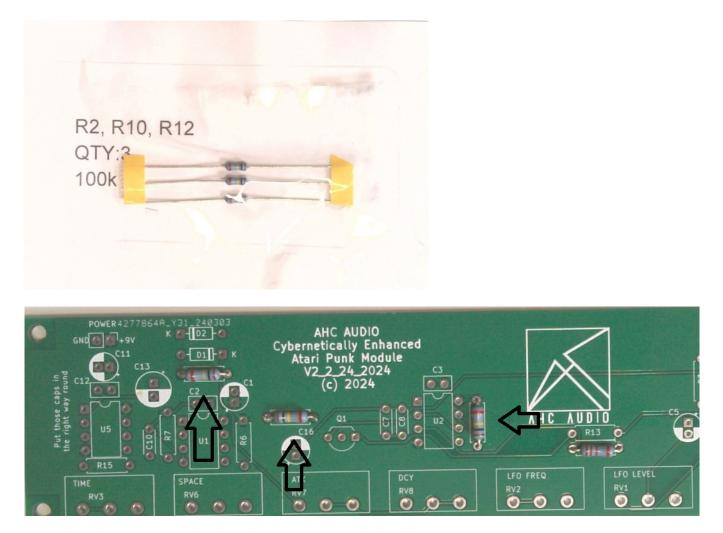
Step six: Bend, place, solder, and trim the ends for R3,R13. These are 1k resistors with color bands Brown, Black, Red, (tolerance).
