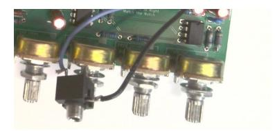
Solder the black wire to the GND on the LINE OUTPUT, and the blue wire to the OUT on the LINE OUTPUT. You'll have to strip the wires. You will want to tin the wires - meaning you strip them, twist the bare strands, and then coat them in solder to prevent stray strands of wire from shorting out nearby terminals.
