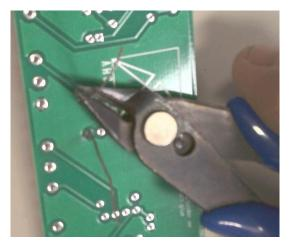
Step five: Bend, place, solder, and trim the ends for R2,R10,R12. These are 100k resistors with color bands Brown, Black, Yellow, (tolerance).
