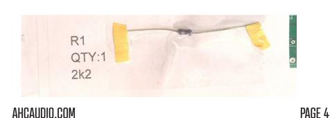
Step four: Bend R1 and place it on the board, in the spot marked R1. Solder it in place, and clip the ends. For all other components, follow these steps - Bend, place, solder, and trim the ends. All of the components will go in through the front side, and all of the components will be soldered on the back of the board. For a soldering tutorial, you can click on the QR code to the right.
