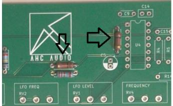
Step seven: Bend, place, solder, and trim the ends for R4,R11. These are 10k resistors with color bands Brown, Black, Black,Red, (tolerance).
