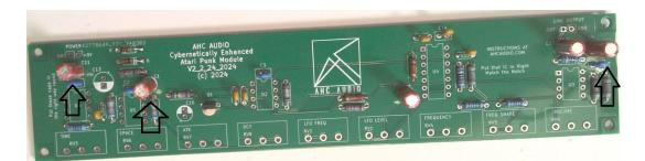
Step seventeen: Warning - this is another polarized component. Place capacitors C5,C17 - 100u - the right way round - solder and clip. Negative stripe goes to white half of silkscreen.
