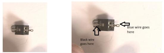
Strip one end of the blue wire and solder to the jack as shown. Note where the blue wire is connected to the jack.
