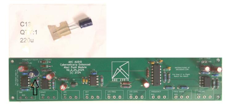
Step nineteen: Warning - this is another polarized component. Place C16, which is a 2.2u capacitor - make sure its the right way around. Negative stripe goes to the white silkscreen half.
