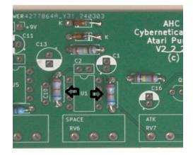
Step ten: Bend, place, solder, and trim the ends for R14,R15,R16 These are 220 ohm resistors with color bands Red, Red,Black,Brown, (tolerance).
