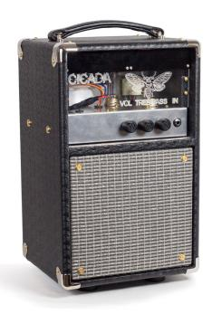
The AHCAUDIO CICADA is a 4 watt tube amplifier. It uses a 5755 tube for the preamp tube and an EL82 tube for the output tube. It has a 6" speaker in a sealed cabinet. The tone controls are a James design providing a wide tonal range for the amplifier. It is constructed using vintage techniques - point to point wiring on a Bakelite custom manufactured turret board.
