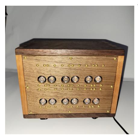
The AHCAUDIO IN1DRT24 and IN1DRT12 are true nixie date/time clocks. There are four buttons on the back, the leftmost one turns the tubes on and off, the center of the reamining three selects the setting to be changed, and the ones on either side of the selected number up and down.Requires a 12V center positive 5.5x2.5 1.5A power supply.
