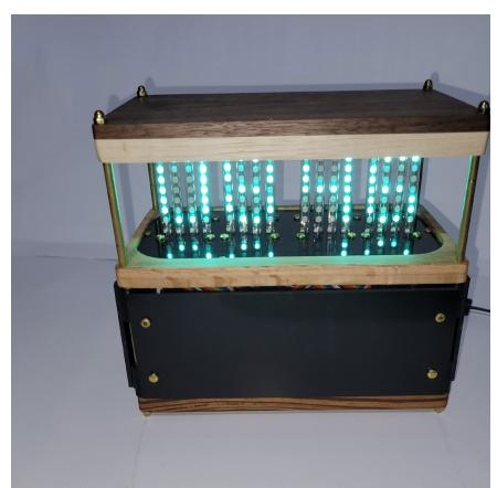
The AHCAUDIO IV26HR12 and IV26HR24 are vacuum fluorescent display clocks. There are three buttons on the back, one turns the display on and off, and the other two increase the hours and minutes respectively. Requires a 12V center positive 5.5x2.5 1.5A power supply.
